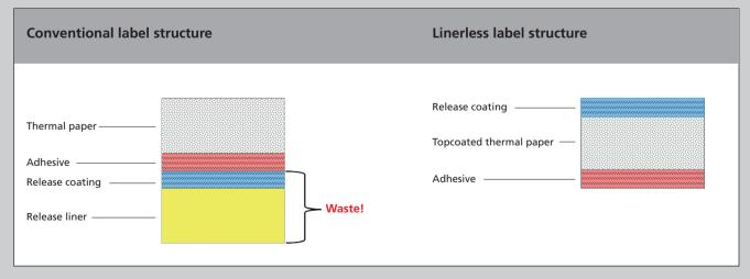
As with adhesive tape, the adhesive layer lies directly on the underlying paper layer.
